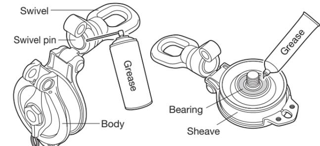
Apply grease to the gap of the swivel pin in the inner side of the body to prevent the rotation failure and abrasion of the swivel.
